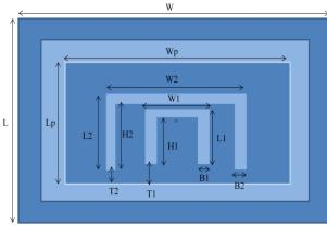
Fig. 4 Geometry of U-slot triple-band antenna
