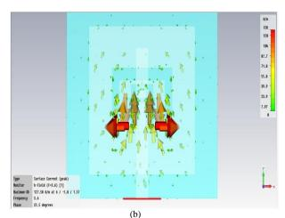
Fig 7 Surface current distribution at 3.6 GHz (a) For U-slot dual- band antenna (b) For U-slot triple- band antenna
