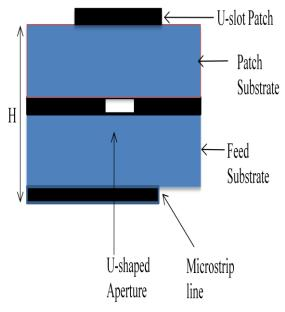
Fig. 1 Geometry of aperture coupled antenna
