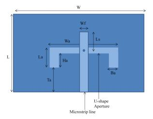
Fig. 2 Geometry of U-shaped Aperture
