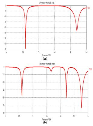
Fig. 5 Return loss (a) U-slot dual band antenna (b) U-slot triple band
