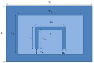
Fig. 3 Geometry of dual-band U-slot antenna
